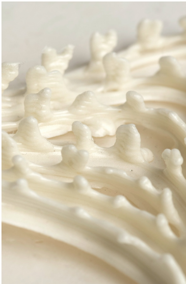
Above Fast setting time surface height inconsistencies
