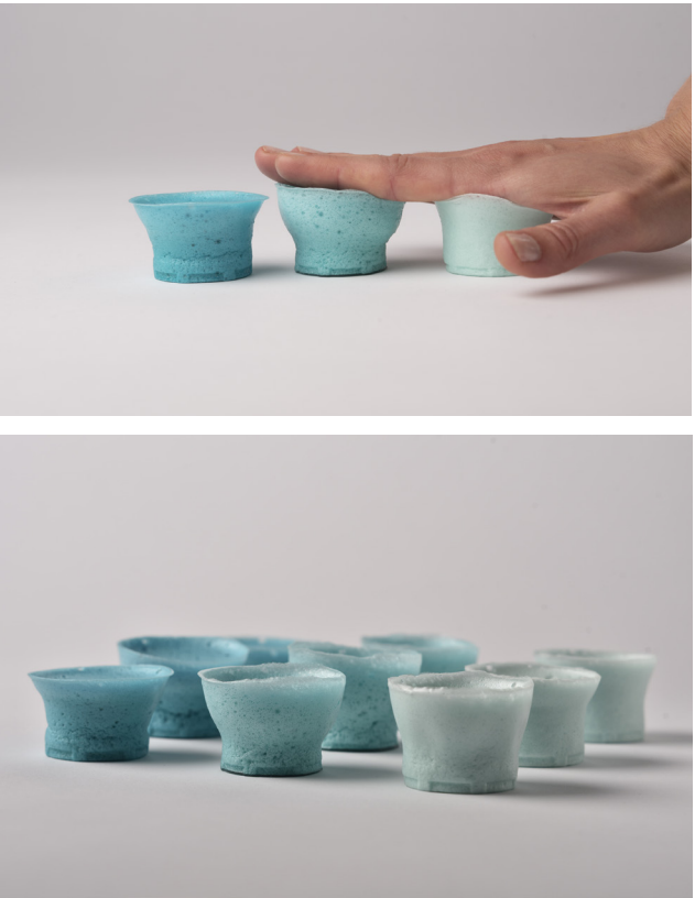
Above Colour-coded samples use natural pigments to visually emphasises gradual increase in the biomaterial's flexibilities
