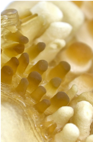
Above Varied shrinkage percentage form distortion
