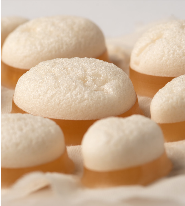
Above Initial experiments with gelatin-based biofoams reveal a clear separation of soft, flexible biofoam and hard, sturdy bioplastic base Gelatin Biofoam: Water 79%, Gelatine 7.5%, Glycerin 12%, Foaming Agent 1.5% Following page R Detail of a heterogeneous gelatin-based biofoam surface with vertical density separation in the front Scale 120 x 120 x 35 mm
