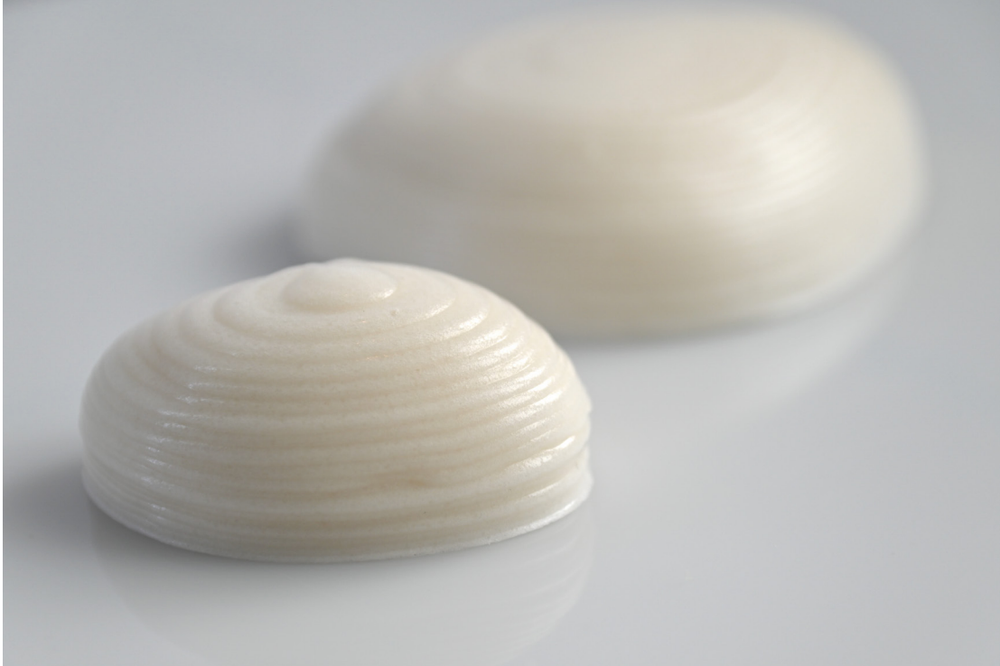
Preceding page and above Freshly printed high-density, low-flexibility agar-based biofoam units are firm and sturdy. Compression is only noticeable in the base layers, however, the overall surface is even and smooth with only subtle layer inconsistencies
