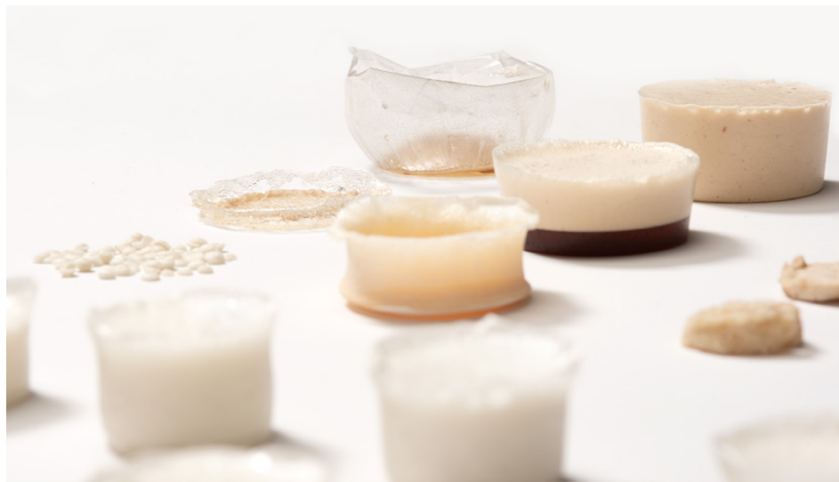
Preceding page and above A collection of biofoam samples demonstrates experiments with different formulas to produce a range of biofoam densities, thicknesses, colours and surface finishes
