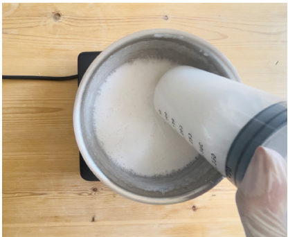
Step 6 Fill up a large syringe with the biofoam while still hot
