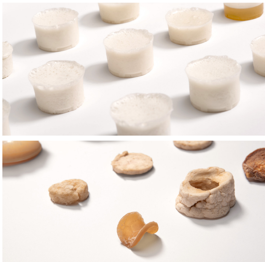
Above and facing page A series of samples demonstrating experiments with a range of foam-making processes. These include the implementation of the chemical reaction between vinegar and baking soda resulting in uneven, high-density foams as well as more consistent homogeneous samples using castile soap
