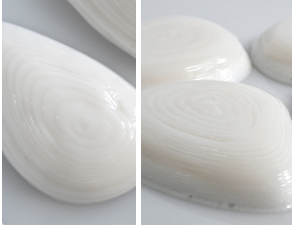
Above Freshly printed medium-density, high-flexibility agar-based biofoam units are very delicate and bouncy. Compression is noticeable in the lower quarter, however, the overall surface is even and smooth
