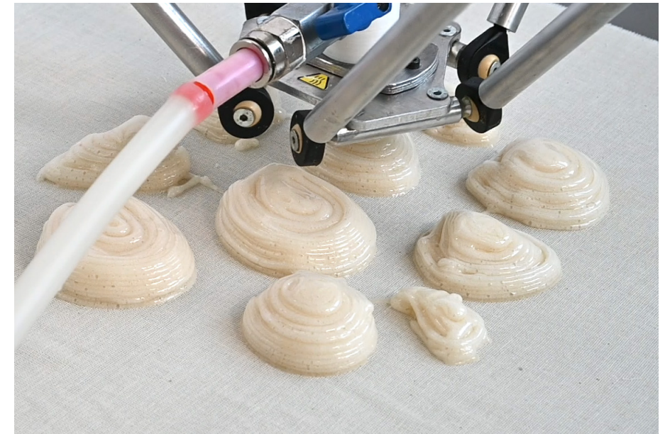
Above 3D printing high-density gelatin-based biofoam with reduced content of water increases the material's homogeneity. This enables more consistent behaviour of the material in combination with refined printing settings
