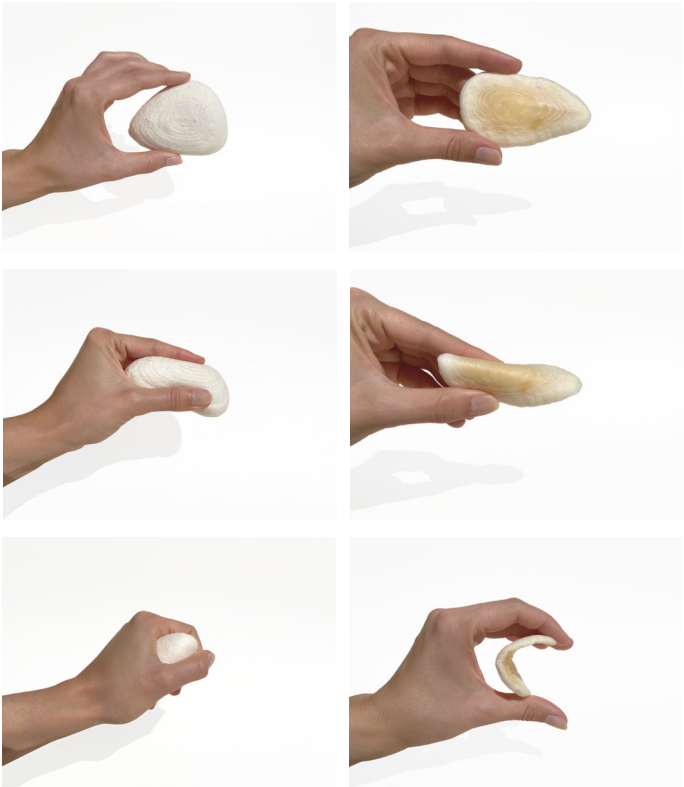
Above Interaction with a range of agar-based biofoam units shows the difference in the densities, flexibilities and thicknesses of the material, achieved through a range of material formulas as well as 3D printing settings
