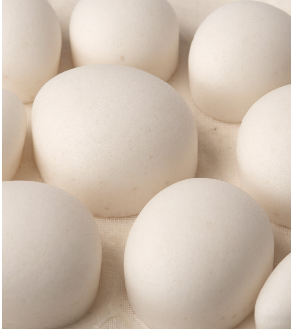
Above Initial experiments with agar-based biofoams reveal homogeneous surfaces with high flexibility and adaptability Agar Biofoam: Water 88.3%, Agar 3.5%, Glycerin 6.8%, Foaming agent 1.5% Following page L Detail of a heterogeneous agar-based biofoam surface with high-density units in the front Scale 120 x 120 x 35 mm
