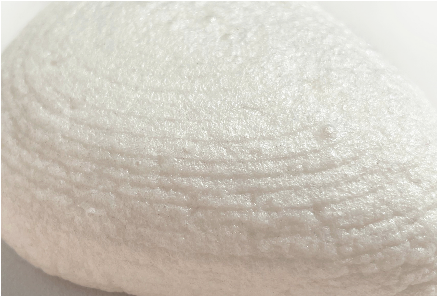
Above Detail of a cured agar-based biofoam unit shows refined layers with a decrease in form inconsistencies due to the biomaterial's shrinkage during the curing process
