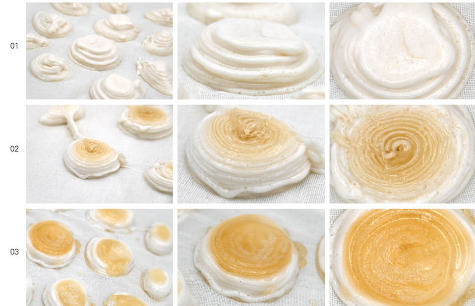
Above Initial experiments printing gelatin-based biofoams reveal inconsistencies in density and flow caused by increasing pressure in the filament tank and separation of the biomaterial's foam and liquid parts. Further observations and experimentations are required in order to incorporate vertical gradients of biofoams in a more controlled manner
