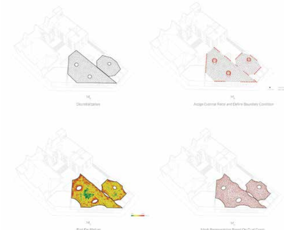
Image 6 The form-finding process of the canopies based on particle spring systems.
