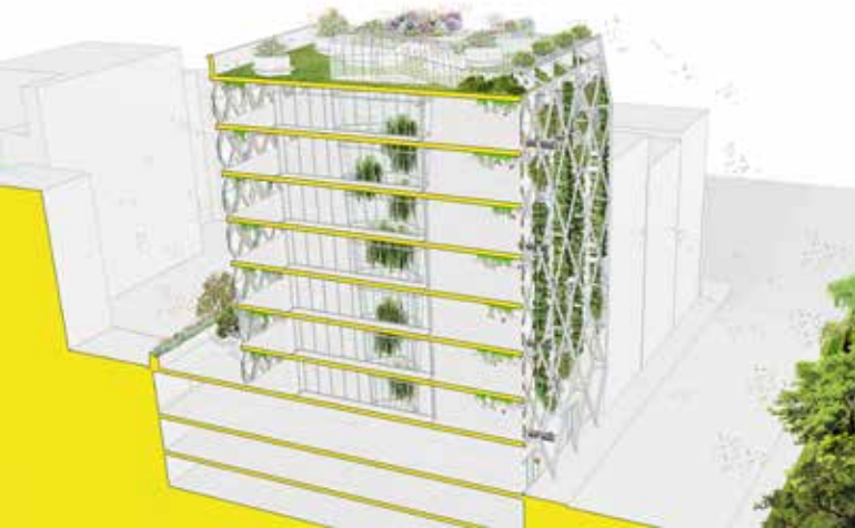
Image 3 Building section perspective mapping the trajectory of butterflies from across the street Petrosino Park through the double-skin facade vertical meadow finally up to the pollinator rooftop garden.
