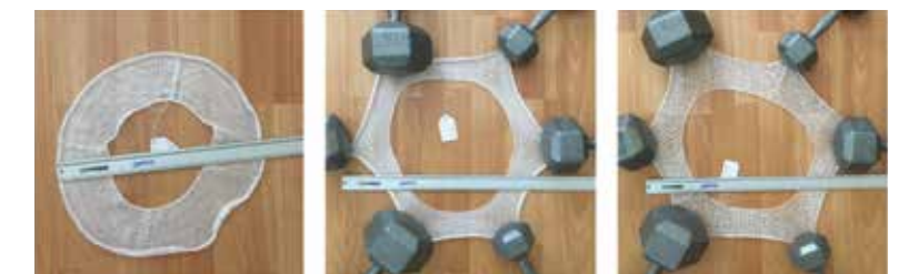
Image 10 Prototypes produced for Lumen to achieve a more nuanced range of stretch factors ranging in size from XS to XL.
