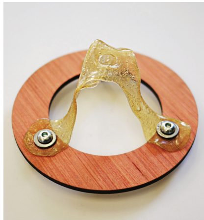
Image 12 (top left) Dried pectin-chitosan composites of 25% pectin with (from left to right) 2%, 4%, and 8% chitosan concentrations Image 13 (above) Three-pronged chitosan tripod made by hydro-forming dried film onto three holed jig
