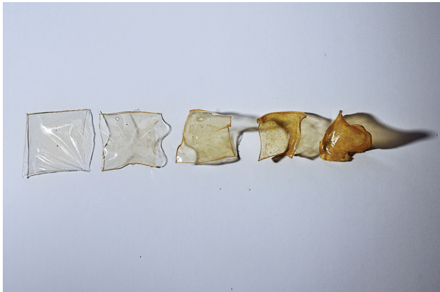
Image 12 (top left) Dried pectin-chitosan composites of 25% pectin with (from left to right) 2%, 4%, and 8% chitosan concentrations Image 13 (above) Three-pronged chitosan tripod made by hydro-forming dried film onto three holed jig
